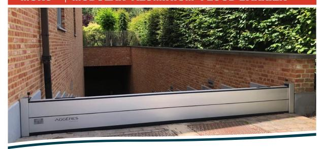
The modular flood barrier consists of stackable, hollow, reinforced aluminium body sections, placed within two U-shaped mounting devices within or in front of a door/gate opening, between walls, etc. The barrier sections are equipped with durable and easily-compressed seals. This flood barrier has already been used worldwide and has proven its effectiveness.
